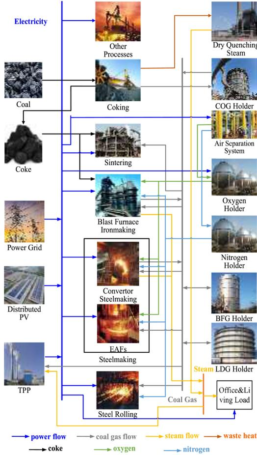
Fig. 1. Typical multienergy system inside an ISP.
