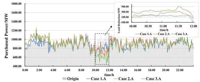
Fig. 4. Load curves in different cases.
